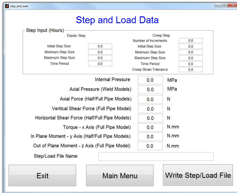
Figure 7.4: The GUI module to create load files. Several different system loads may be applied. Load step durations and parameters used in FEA analyses may also be defined here.
