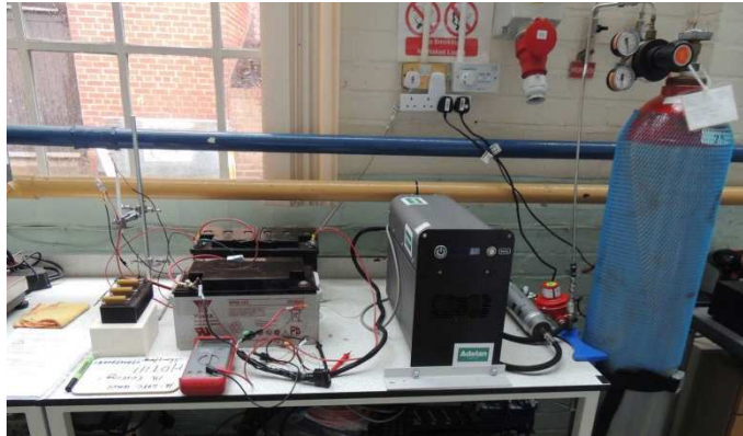
Figure A4-1 UoB micro-tubular SOFC test set-up
