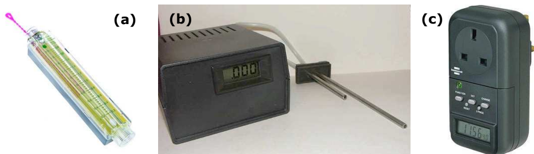
Figure 5-6 Photographs of (a) 0.2 to 2 L.min -1 Parker Liquid Flow Indicator, (b) desiccant solution density meter, and (c) Brennenstuhl PM230 electricity monitor
