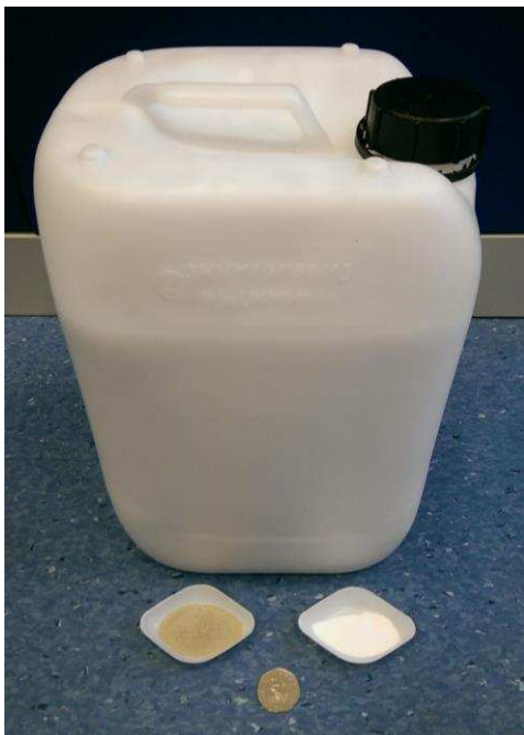
Figure 6 Photograph of the barrel containing a suspension of MIL-53(Al) formed by continuous flow in our scaled-up reaction (centre), together with a commercial sample (bottom left) and dried MIL-53(Al) from the barrel (bottom right). A fifty pence piece is shown for scale (bottom centre).
