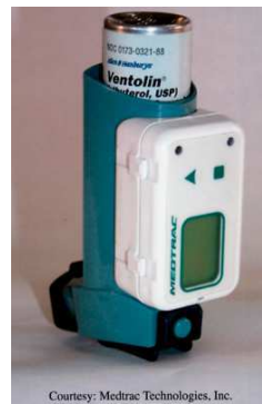
Fig.(2). An MDILog device (white box) attached to the back of a normal metered dose inhaler (MDI) [27] (image included with permission from Elsevier).
