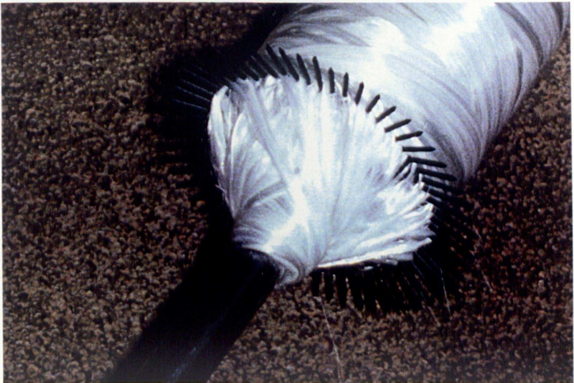
Fig. 8.4: End cap used to prevent fibre slippage at turnaround
