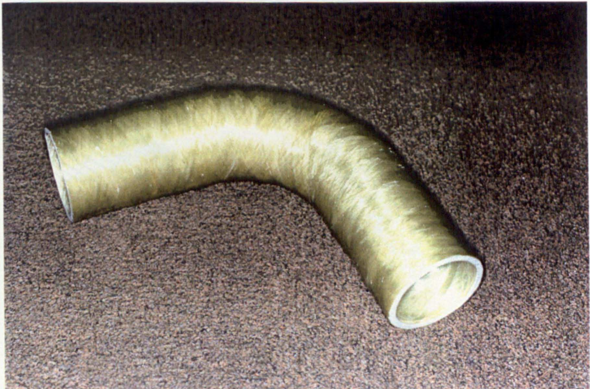
Fig. 8.14: Typical finished elbow after removal of turnaround regions and washing-out of plaster mandrel
