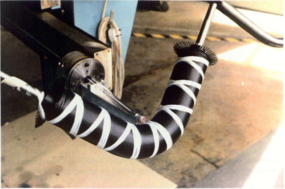
Fig. 8.13: Dry winding of an elbow on a dummy mandrel to demonstrate fibre paths
