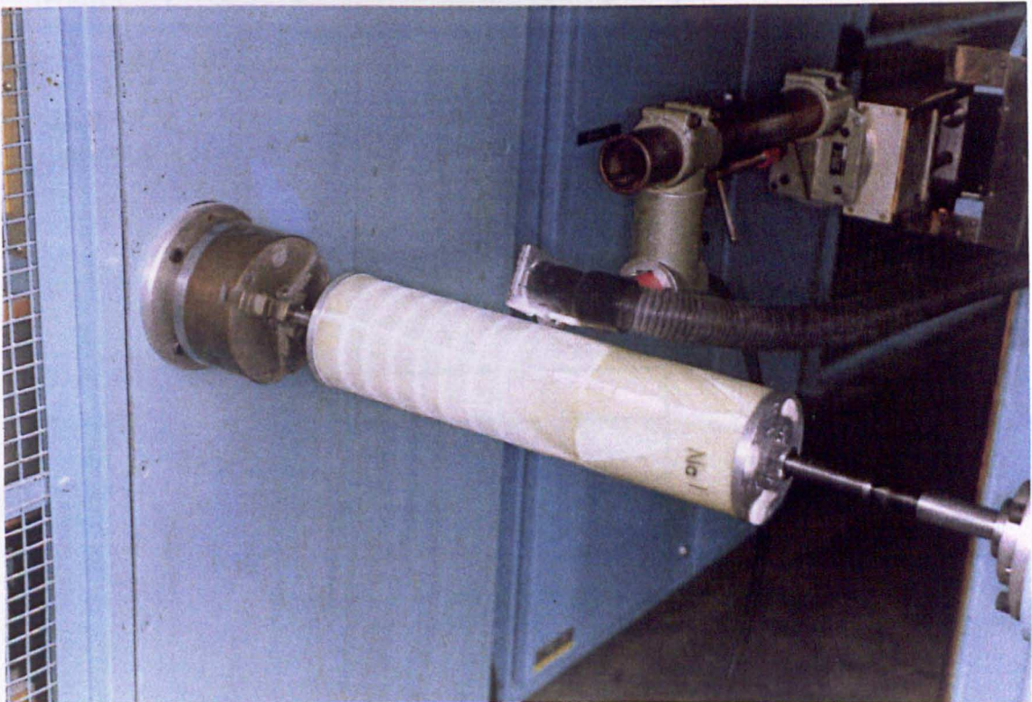
Fig. 5.7: Slicing of typical specimen ( \pm 30^\circ winding angle) into rings using a diamond saw driven by an air turbine
