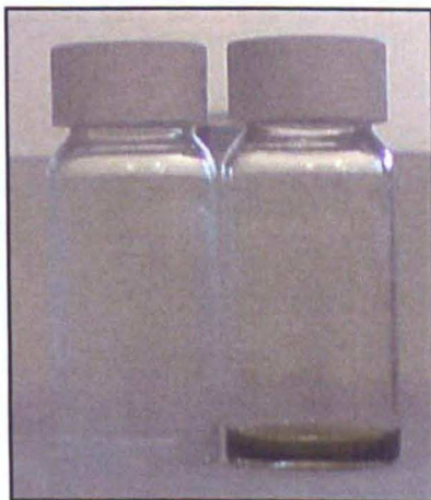
Figure 5.18: Enzyme activity was not detected with PLGA particles (left in the image) but was marked by a colour change of the TMB substrate to dark blue/green in the presence of PLGA-HRP particles.
