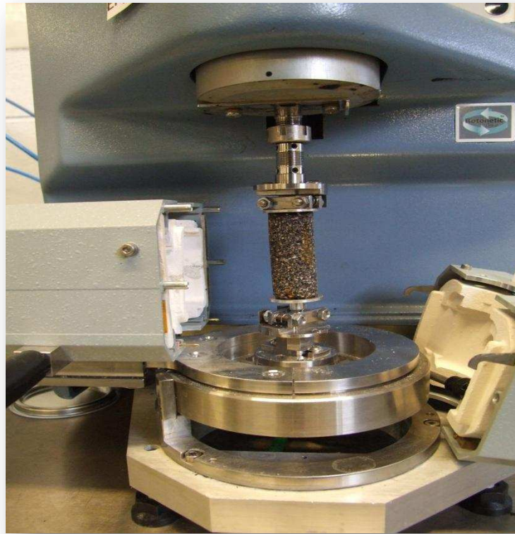
Figure 4 Sample installation in the Gemini ETC
