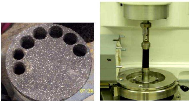
Figure 2.22 Cored specimen and sample mounted in the DSR (Zollinger, 2005)
