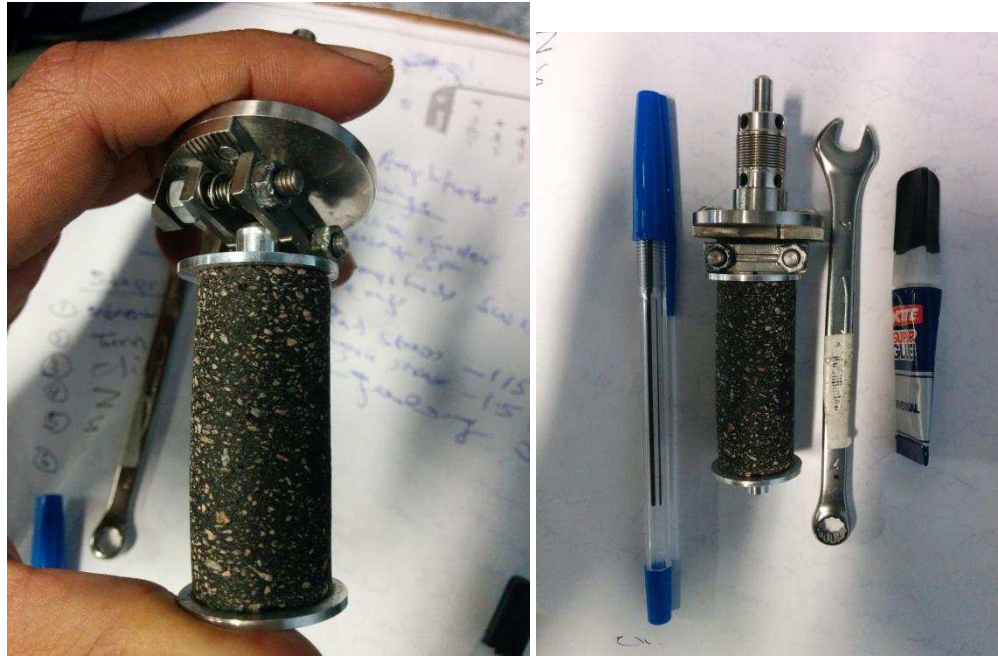
Figure 3 Fixing glued sample to solid fixture
