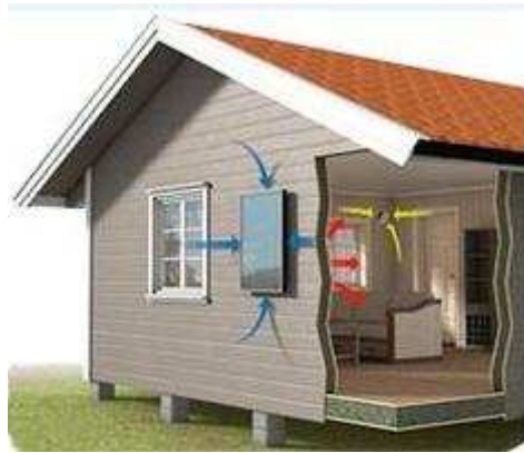
Figure 2.3.2 A schematic diagram of solar thermal air collector application on a single family house (SolarVenti, 2015)
