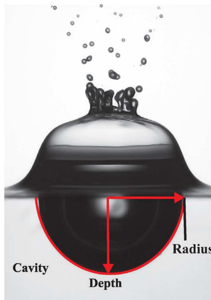
Fig. 2.9: Visualization of the cavity for a acetic acid drop impact onto a deep liquid pool (Shadowgraph from Bisighini (2010)): We = 2177 , Fr = 691 , Re = 12642
