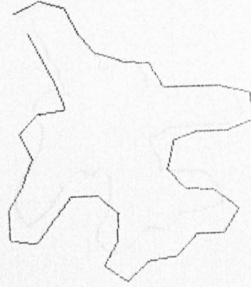
2. Contour around aeroplane normalised to 100 vectors
