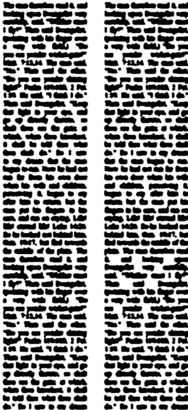
Figure 3: Knuth-Plass layout (left) versus a first-fit algorithm (right). The text has been greeked to draw attention to layout rather than content. Note that Knuth-Plass results in looser spacing of certain lines where it helps avoid extremely loosely-set lines ahead. Even without using hyphenation (this implementation of Knuth-Plass does not include a hyphenation algorithm) the differences are pronounced.
