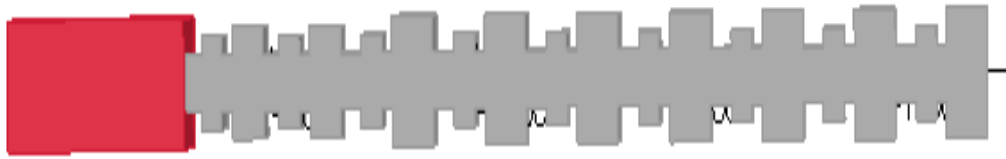
Figure B-1: Detail of the choke used for the scale up system. The resistive choke is in red colour and is situated at both feed and the discharged ends while the reflective chokes are connected close to the applicator
