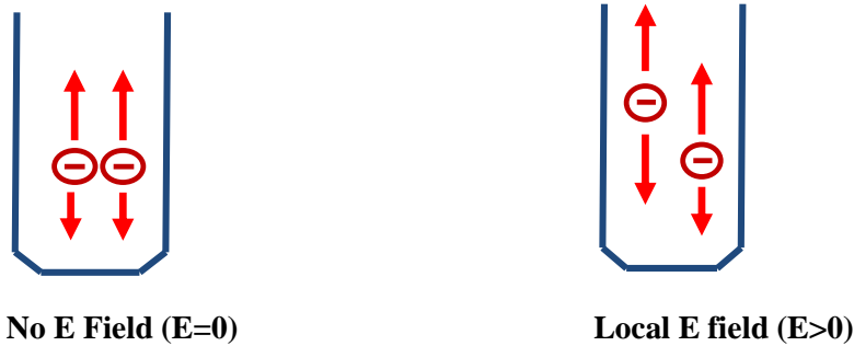
Figure 3-3: Charged Particle following the Electric Field (Lidstrom et al., 2001)
