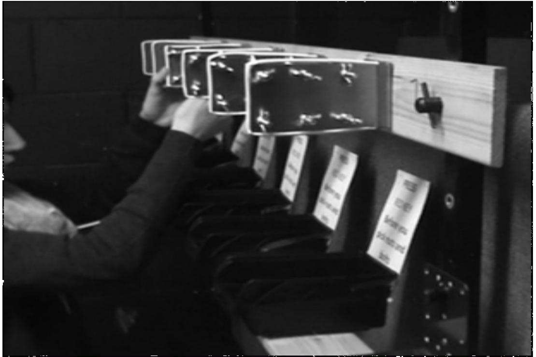
Figure 5.3 A: Performing assembly at above shoulder height
