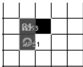
FIGURE 5.19: A case where the GRUE agent has moved horizontally and lined up with its target hole. The hole is right next to the agent, as is an obstacle. The Fill Hole program is removing the horizontal direction, and creating a down direction instead. If the Avoid Obstacle TRP runs and assumes the agent is still moving to the right, it can have the effect of moving the agent onto the target a cycle early.
