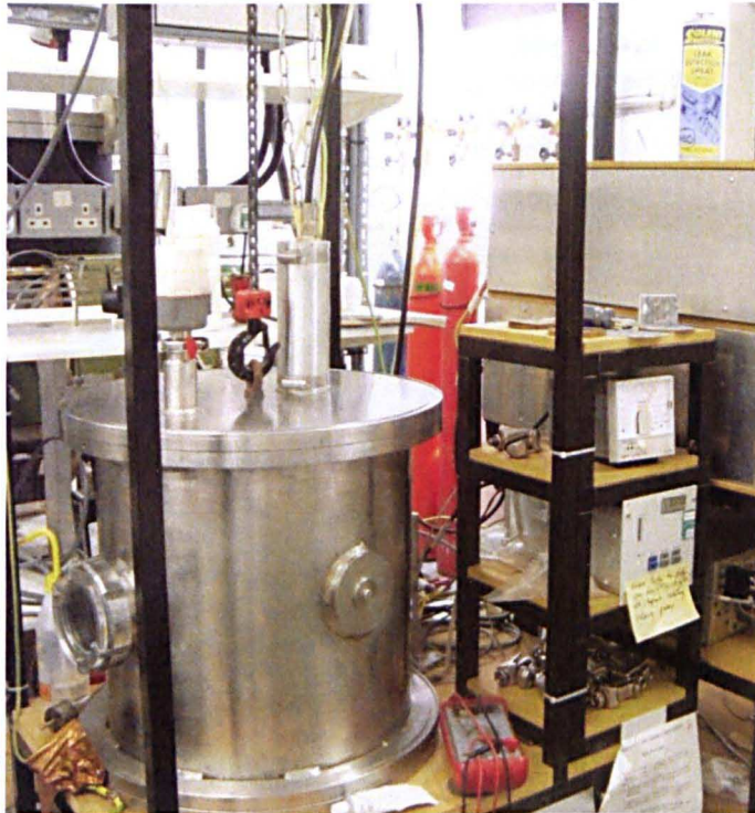
Figure 2.24. PVD Deposition Chamber, Nottingham University.
