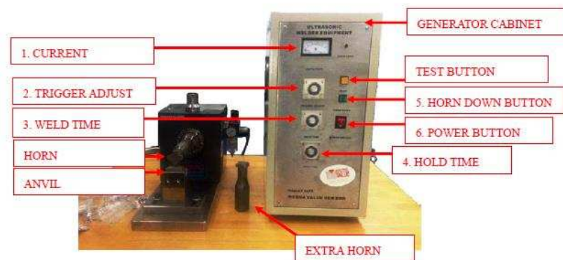
Figure 3-16 The ultrasonic welding machine
