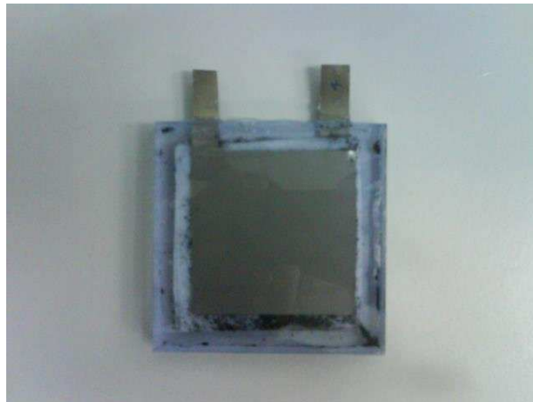
Figure 4-3 Supercapacitor cell Cap-2
