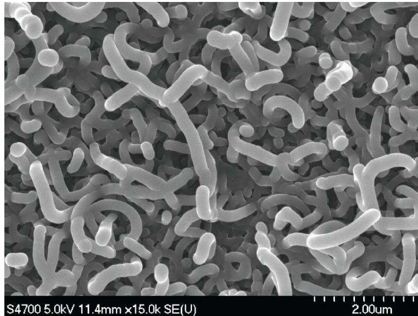
Figure 2-4 SEM image of entangled mat of carbon nano tubes [53].
