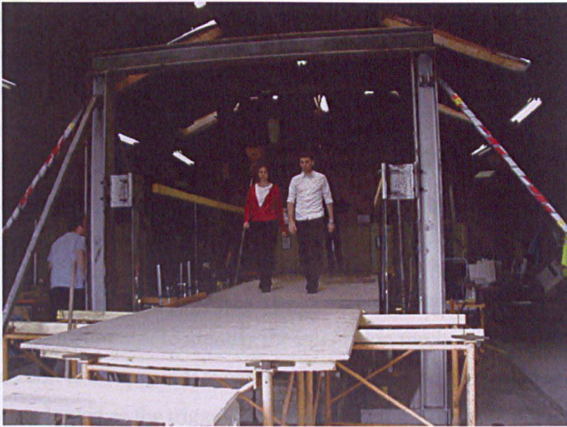
Figure 2.20: Laboratory based platform tests carried out by Sétra as part of the investigation into the dynamic behaviour of the Solférino footbridge, after [27].
