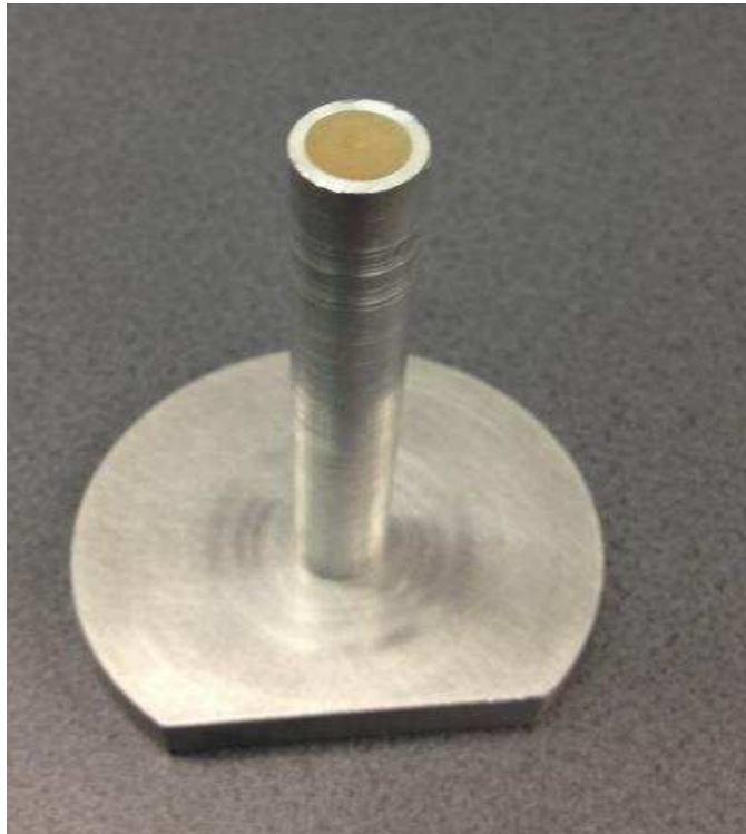
Figure 3. 10: Photograph of a 5mm sample holder.
