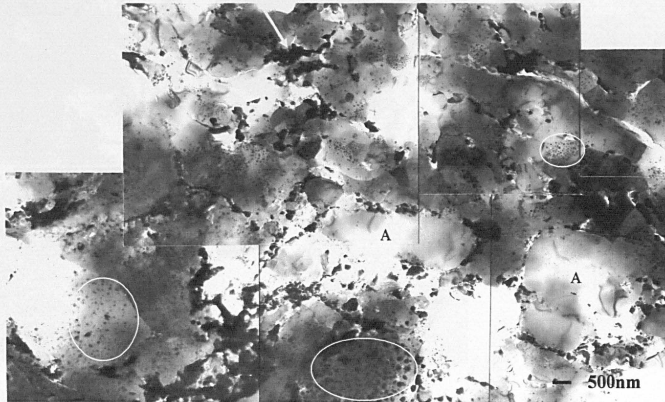
Figure 7.17 TEM montage of the Al 2 O 3 Sn 3 Si coating annealed at 300°C for 1 hour.
