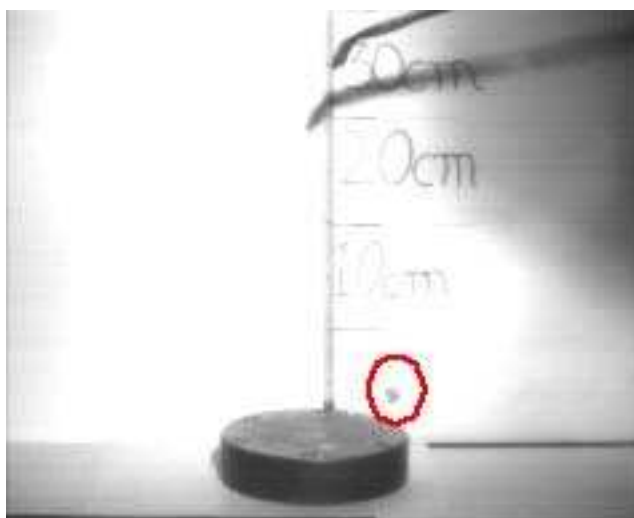
Figure 56: The limestone particle highest position from rebounding to the steel surface.
