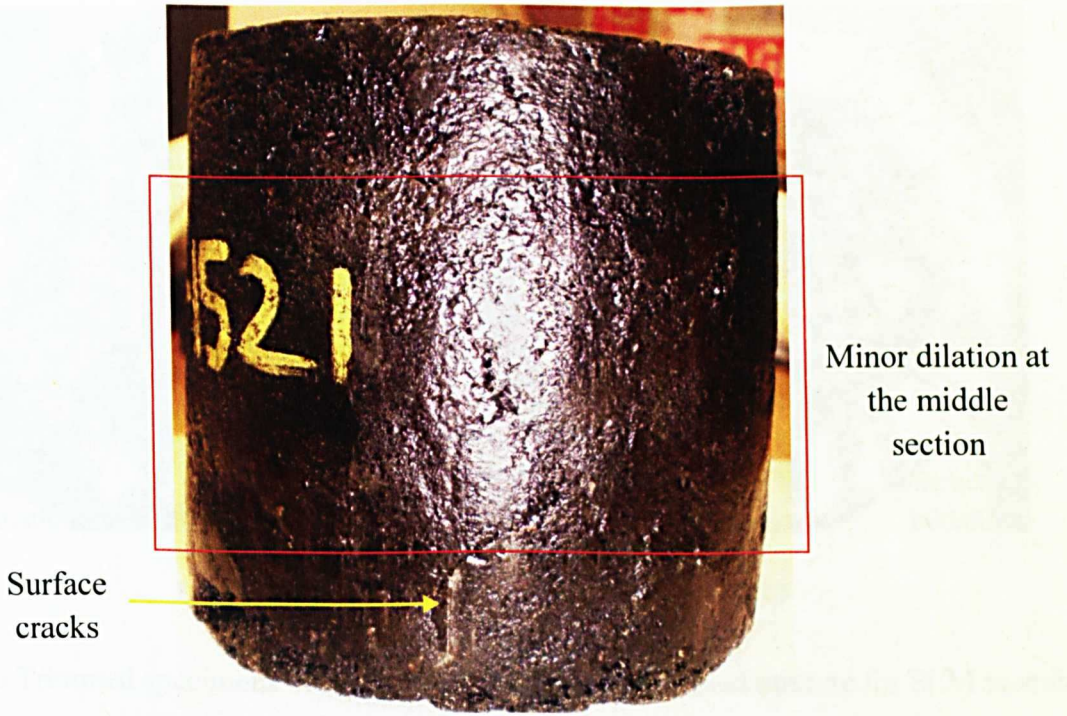
Figure 7.4 Deformed specimen at of the control mixture (test stopped at peak stress)
