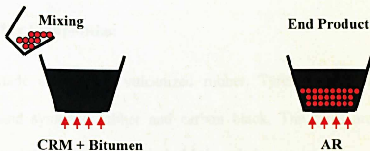
Figure 2.1 Wet process method
