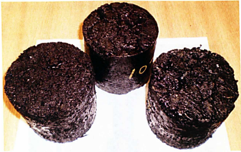
Figure 5.16 Specimen ready for compression testing
