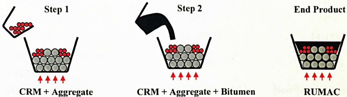
Figure 2.2 Dry process method
