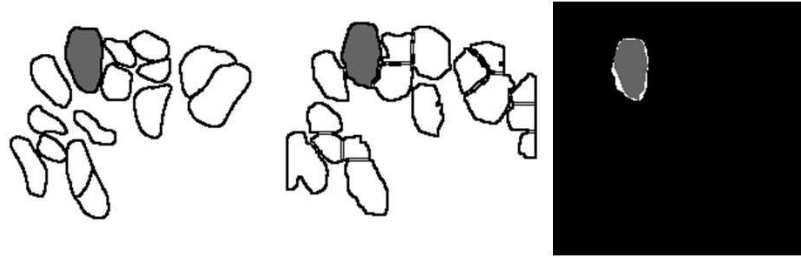
FIGURE 4.7: The illustration of the Dice coefficient evaluation. The left image is ground truth, the middle image is the segmentation result and the right image is the evaluation result. The grey labelled nucleus in the left and middle image is the evaluated one. The grey labelled pixels in right image denote the overlapped pixels between the ground truth and the segmentation result. The white pixels together with grey pixels in the right image denote the union pixels. Therefore, the Dice coefficient is the grey pixels in the right image, divided by the union pixels.
