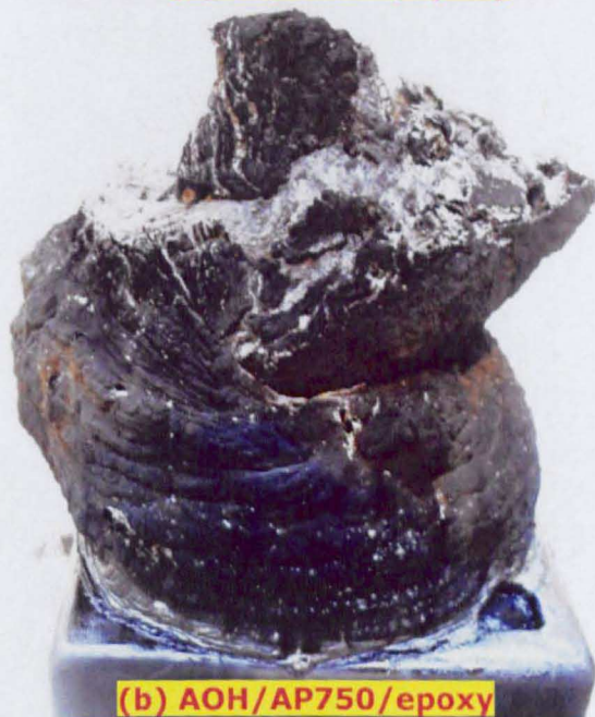
Fig. 10.18: The intumescent action of multi-component epoxy based on: (a) HA, and (b) AOH nanoparticles
