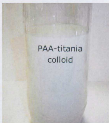
Fig. 6.3: Sterically stabilized PAA-titania colloid in water after one month, (Non stabilised TiO 2 would drop to the bottom within minutes of production)
