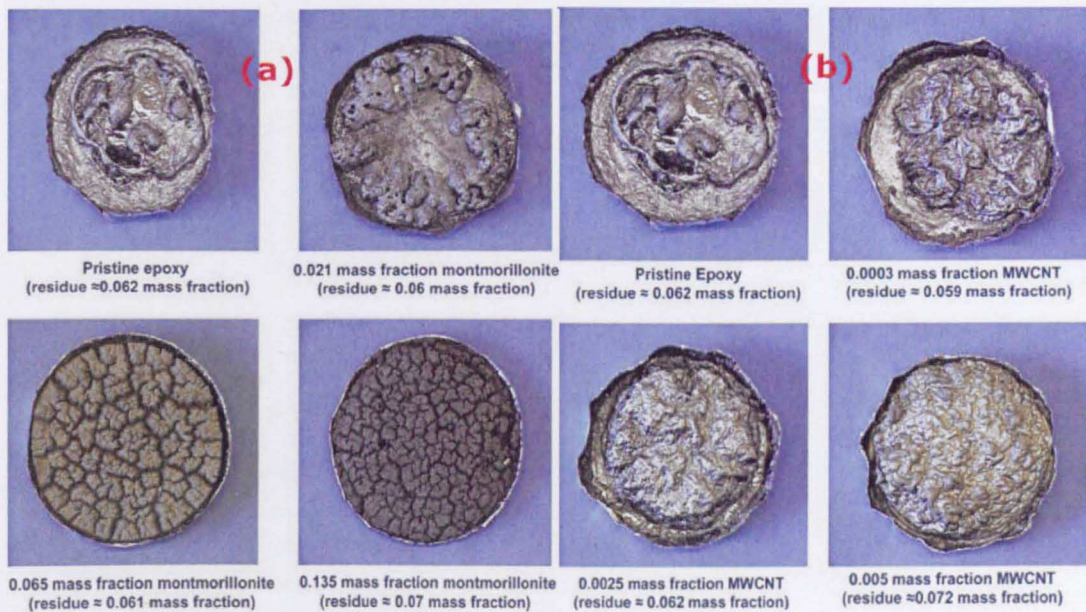
Fig. 2.35: The residue integrity of: (a) epoxy/OMMT, (b) Epoxy/MWCNT, adapted from (Rahatekar et al., 2010)
