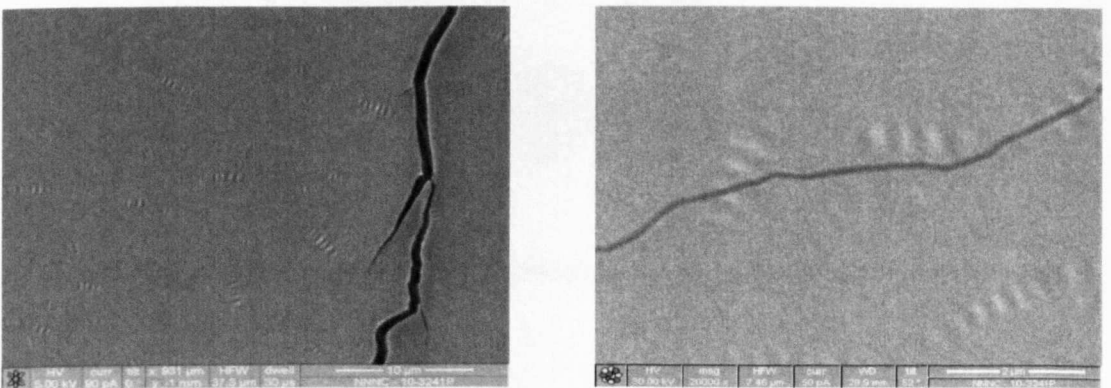
Figure 5-25: (a) Electron micrograph of bitumen D showing an aborted secondary crack. (b) Electron micrograph of bitumen D showing cracked bee-like structures.
