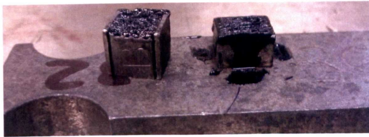
Figure 6-24: Profile photograph of a fractured Vialit pendulum sample (bitumen A)
