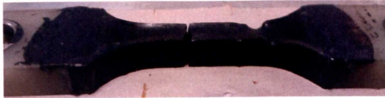
Figure 6-8: Profile photograph of a fractured, healed and re-fractured DTT sample. Note the two crack trajectories: the healed crack near the right end-tab, and the central re-fracture.
