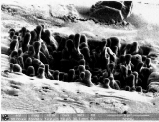
Figure 5-37: (a) Micrograph of peripheral effects of ion bombardment of bitumen D at 3nA and 0° incidence. (b) Image of the effects of ion irradiation in bitumen D at 3nA and 20° incidence.
