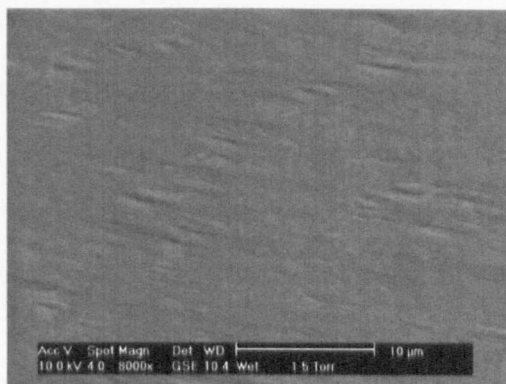
Figure 5-14: Image of bitumen D (aged) at 0°C after the thermal cycle (0°C to 25°C to 0°C).
