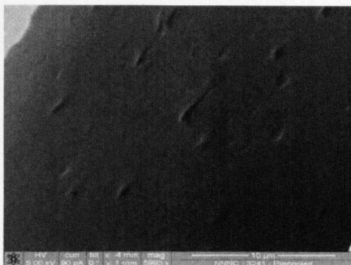
Figure 5-27: Electron micrograph of near-surface bee-type structuring in bitumen D at a crack.
