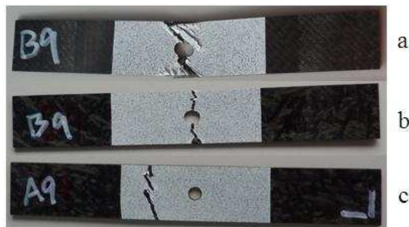
Figure 3-5 Examples of tested notched specimens (37.5mm wide, \varnothing 9\text{mm} hole). (a) NCF with net-section failure; (b) DCFP with net-section failure; (c) DCFP with gross-section failure.
