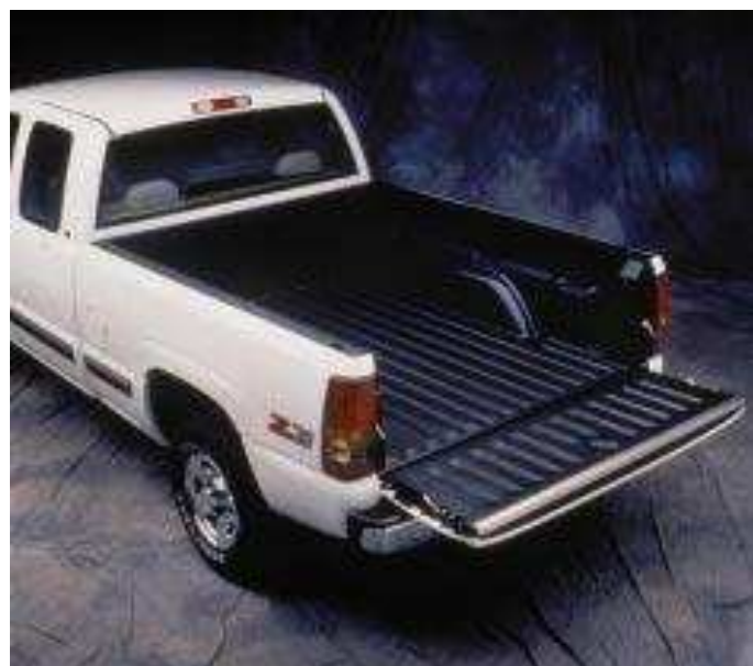
Figure 1-2 Composite truck bed installed in Chevrolet Silverado.
