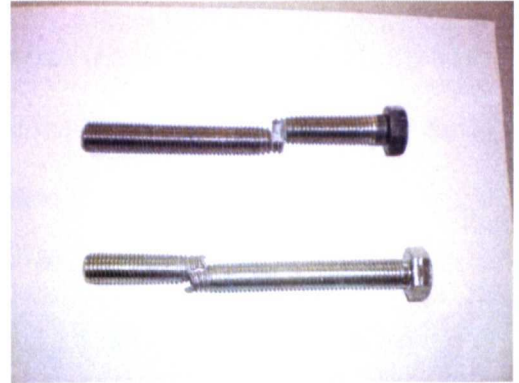
Figure B2 Bolt shank fracture after test
