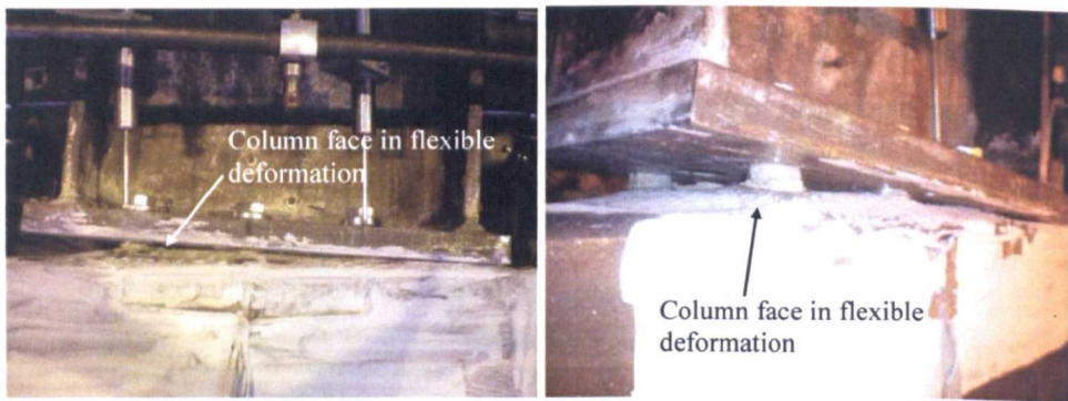
Figure 4.2 Representative deformation mode of connection category II
