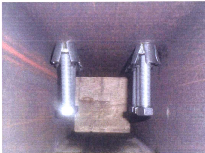
Figure 3.3 Tightened blind bolts in SHS column
