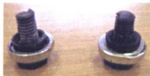
(b) Failure mode of bolt fracture
