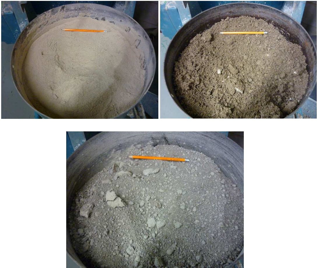
Figure 12: Blending of artificial laboratory soil samples prior to compaction
