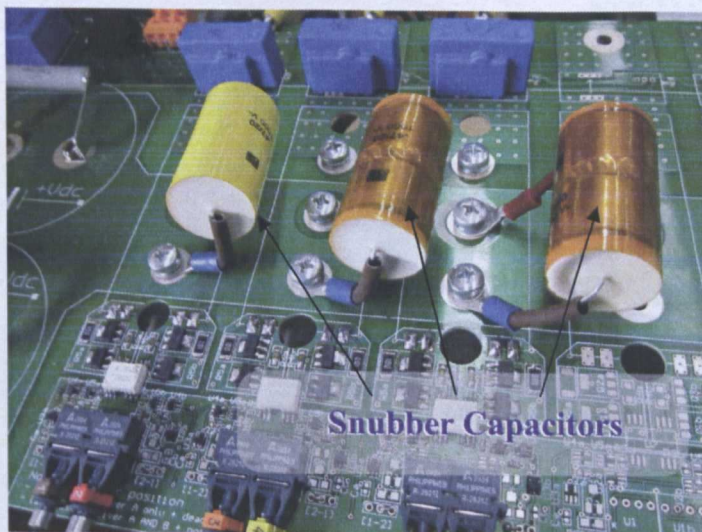
Fig A8 snubber capacitors for circuit protection
