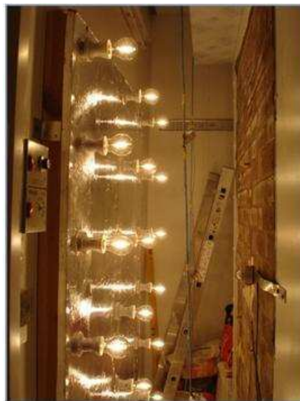
Figure 7-14 - Thermal Chamber - Solar Lighting Board
