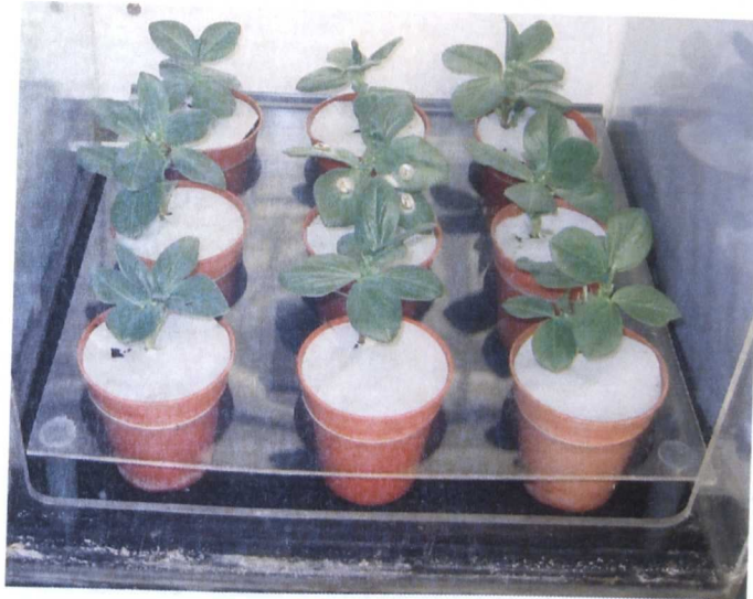
Figure 6.1a Perspex cage with Perspex frame (plan view) containing nine 15-day-old Vicia faba plants.
