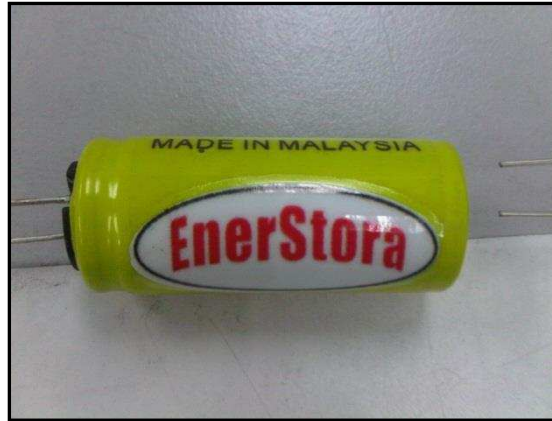
Figure 2 Fabricated Supercapacitor - Enerstora
