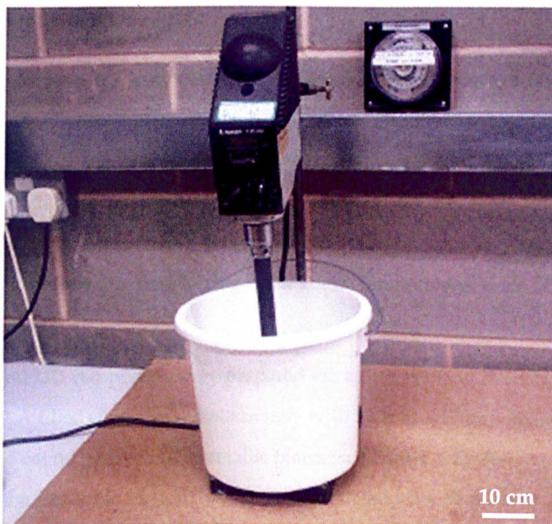
Figure 3-3: Laboratory setup for preparing phosphate glass fibre random mats.
