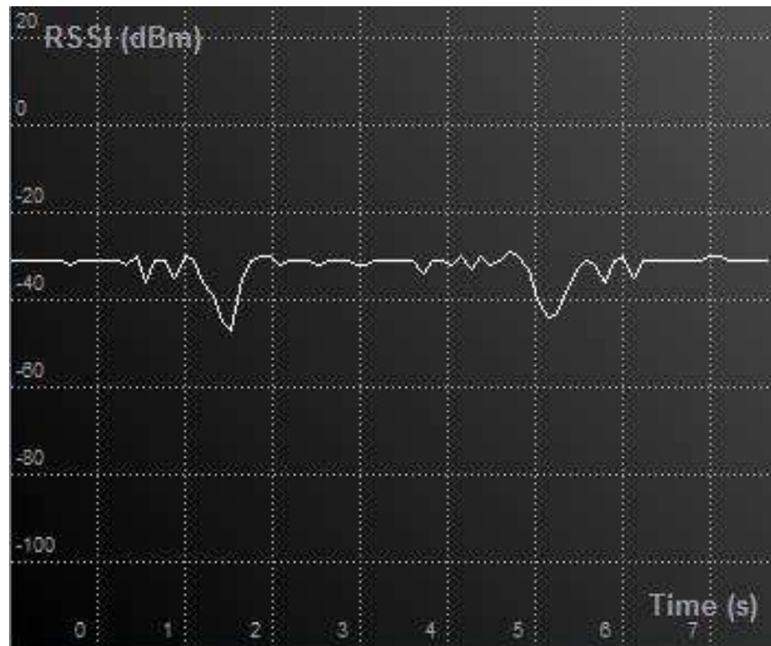
FIGURE 6-17: CHANNEL 0, 0 DBM, 58 KHZ AND A PERSON CROSSING THE LOS TWICE
