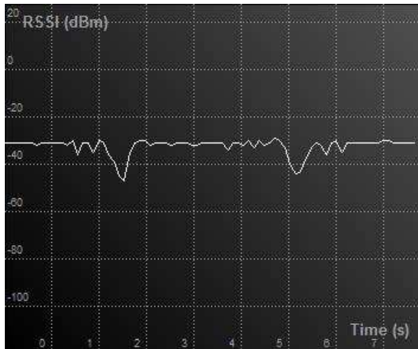
FIGURE 6-12: CHANNEL 0 WITH A 0 DBM INPUT SIGNAL AND A PERSON CROSSING THE LOS TWICE
