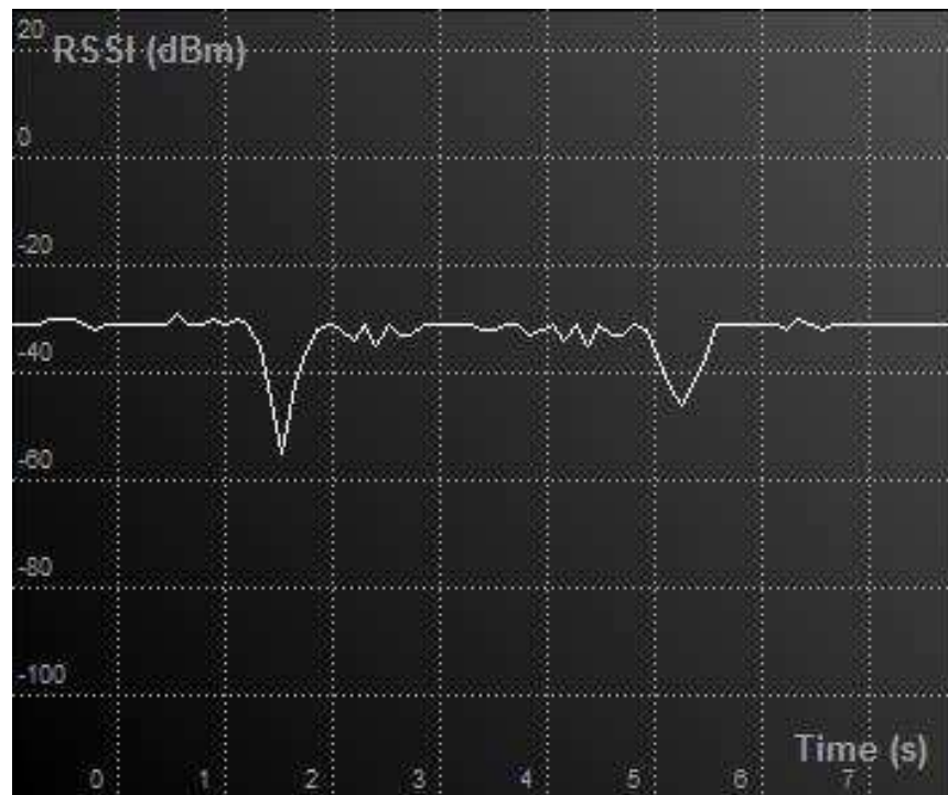
FIGURE 6-7: CHANNEL 255 WITH A 0 dBm SIGNAL AND A PERSON CROSSING THE LOS TWICE
