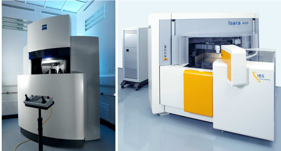
Figure 2.4: The Zeiss F25 micro-CMM (left) and the IBSPE Isara 400 Ultra Precision CMM (right – courtesy of IBSPE).
