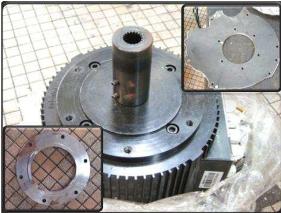
Fig 42: Electric Motor with coupler (center), custom made adaptor plate (top right) and a spacer (bottom left).
