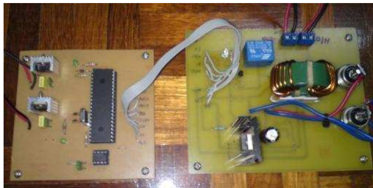
Figure 4: Boost Converter with control circuit.
