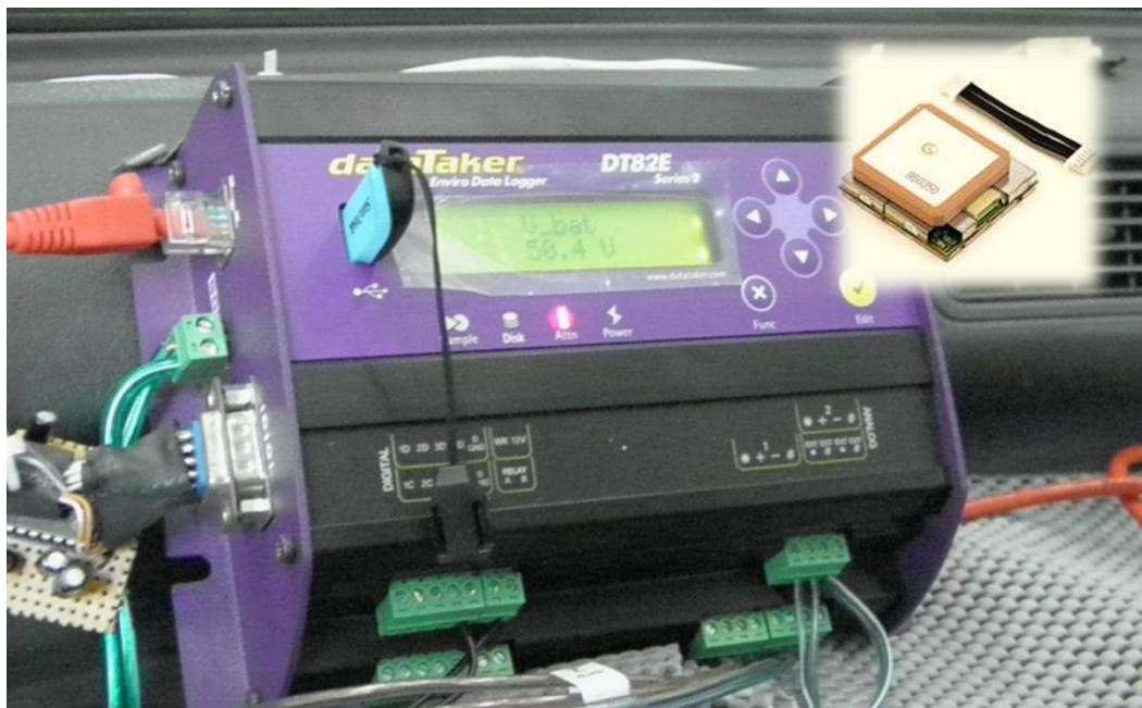
Fig 52: DataTaker DT82E Data logger with flash USB storage logs battery pack current and voltage, supercapacitor current and voltage, GPS timestamps as well as GPS speed.
