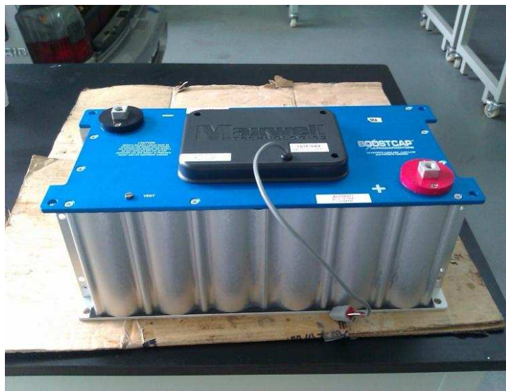
Fig. 46: BMOD0165P048; 165F, 48.6V supercapacitor which weighs 15kg
