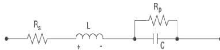
Fig 8: 1 st Order Model of the Supercapacitor
