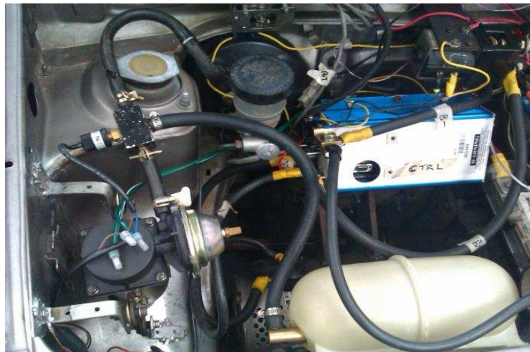
Fig 50: Electric Vacuum Pump (left) connected to the vacuum reservoir on one side and the brake booster on the other. A pressure sensor turns the pump on and off depending on the set level.
