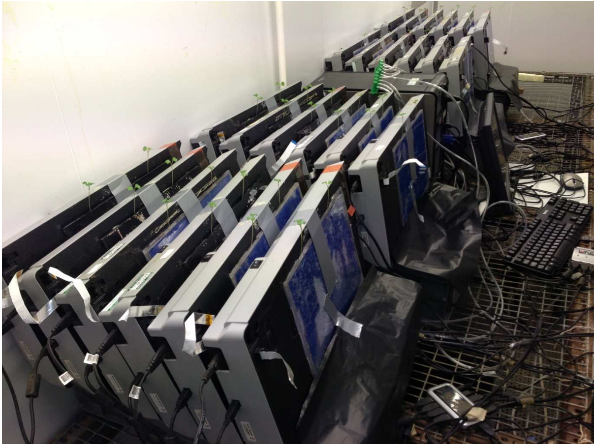
Figure 4.1: The phenotyping platform comprising 24 scanners assembled in four banks of six scanners.
