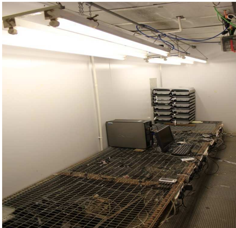
Figure 2.2: Growth chamber showing light source and wire grid on which the scanner banks were assembled.
