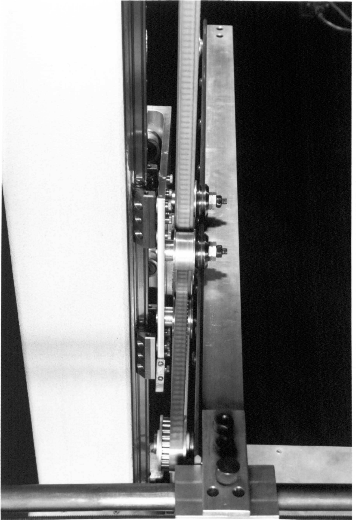
Figure 4-5: A Photograph of the CNC Carriage
