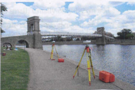
Figure 4-3 The two riverside reference receivers Ref1 on the right and Ref2 on the left with the Wilford Bridge in the background
