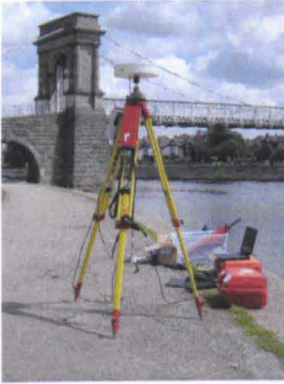
Figure 9-11 The reference receiver for the bridge trial, located on the bank of the river, with the Wilford Suspension Footbridge in the background.
