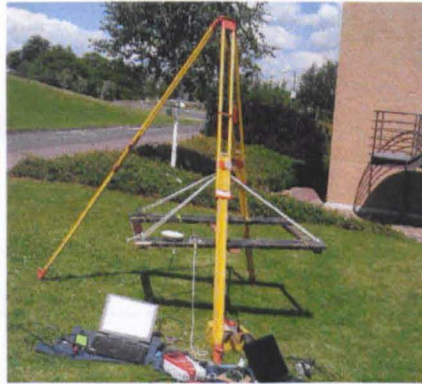
Figure 9-5 Bungee test rig on which an accelerometer is located along with an AT502 GPS antenna attached by a splitter to a JNS100 and a Leica receiver.
