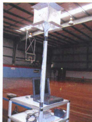
Figure 11-27 The Locata rover with specially designed multipath mitigating antenna
