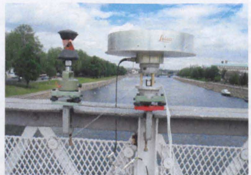
Figure 4-4 The total station 360° prism located next to the GPS antenna and accelerometer
