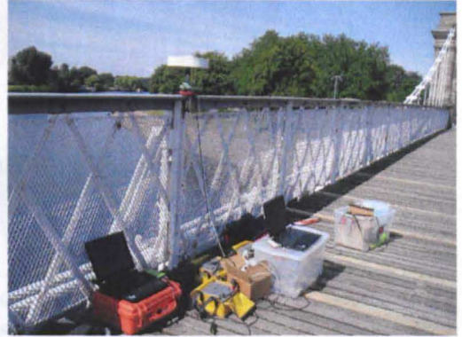
Figure 9-12 The rover station located at the mid span of the Wilford Bridge. The AT503 antenna is connected via a splitter to both the JNS100 and Leica receivers. The accelerometer is strapped to the bridge handrail next to the GPS antenna.
