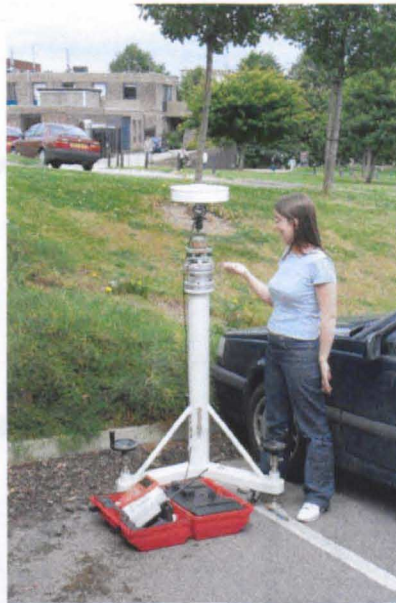
Figure 4-15 The GPS antenna and the total station prism housed together as one unit on a monument.
