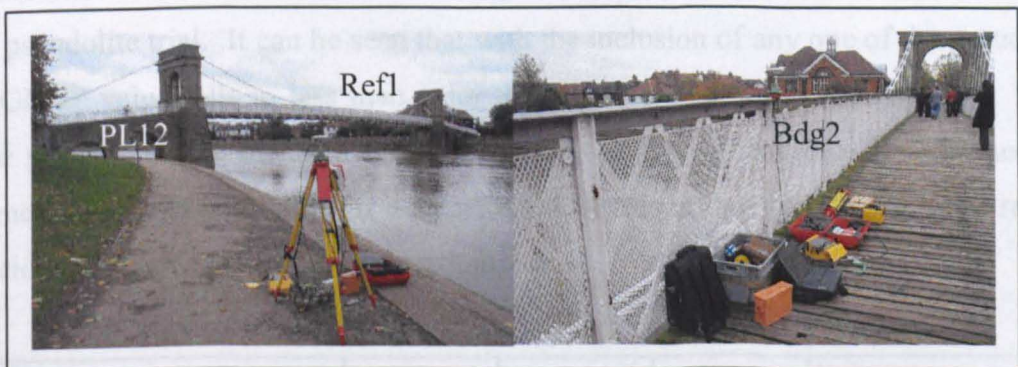
Figure 11-3 The receiver locations. At both Ref1 and Bdg2 there was a Leica dual frequency receiver and an Allstar GPS/pseudolite receiver connected via a splitter to an AT502 antenna.
