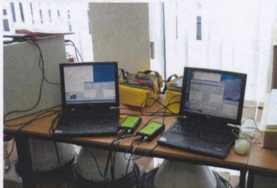
Figure 9-2 The two JNS100 receivers connected to recording laptops, during the zero baseline trial.
