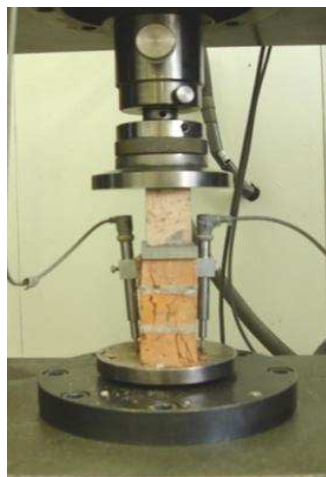
Figure 4.12 The uni-axial compressive strength test of the brickwork
