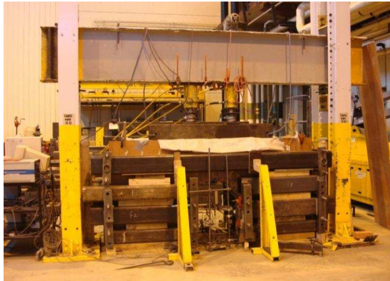
Figure 3.9 Loading system installation for uniform load
