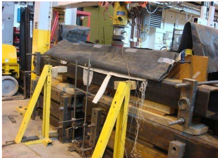
Figure 3.12 Loading system installation for concentrated load
