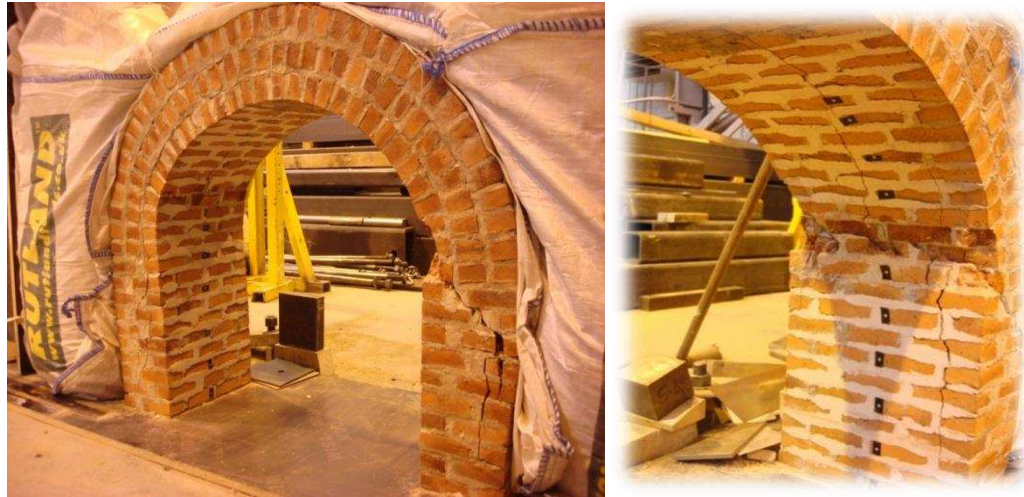
Figure 3.22 (a) Shear failure at sidewalls; (b) Crushing phenomenon at the arch springing
