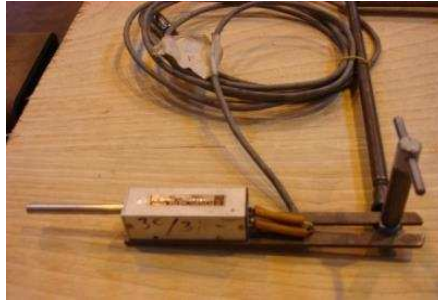
Figure 3.16 Potentiometer with 30 mm range
