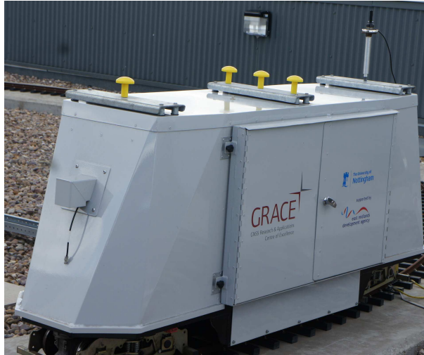
Figure 5.3 – Mounting of Locata antenna on a train during the kinematic trials
