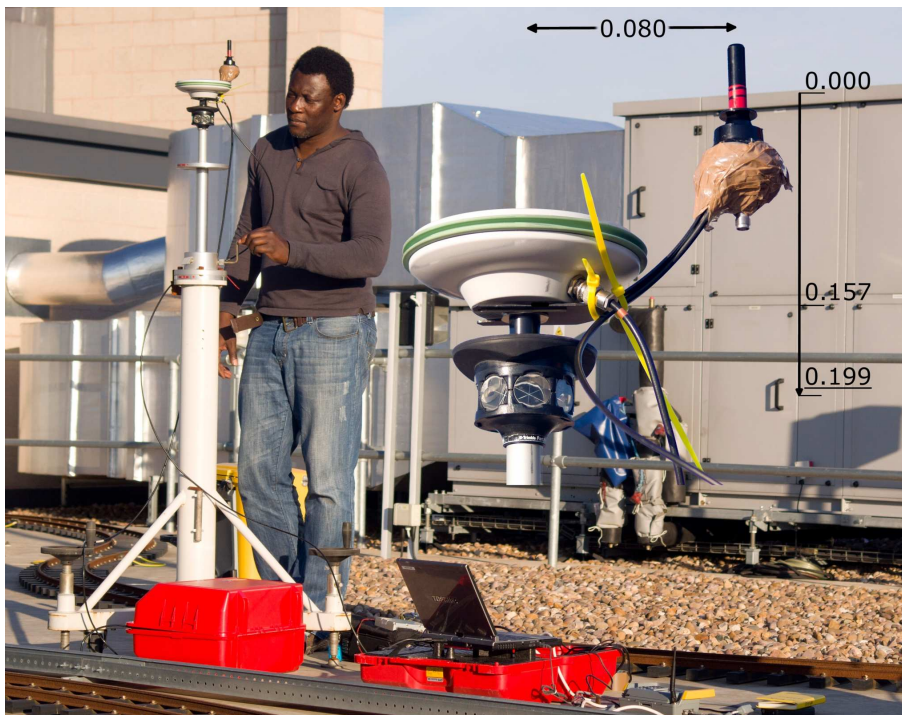
Figure 7.6 – The LTM experiment set-up with Locata HG2403U and Leica GS10 antenna on 360° prism
