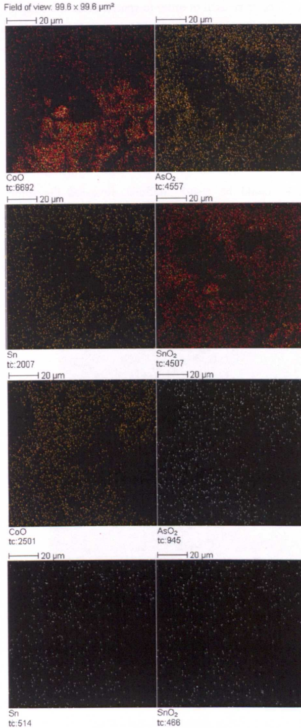
Figure 6.29 Positive Ion High Mass Resolution Results for Selected Trace and Minor Elements in Th153 and Am2.
