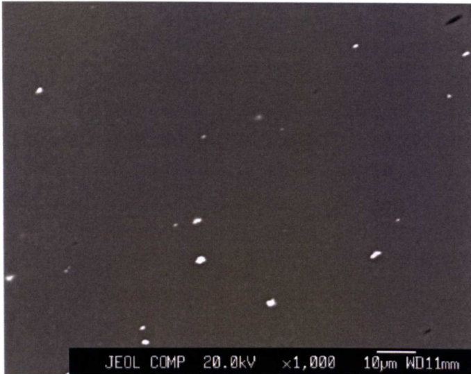
Figure 5.20 BSE Image Showing Small (1–3µm), Scattered Inclusions in a Sample of Semi-Translucent Glass.
