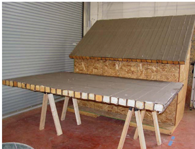
Figure 2.9: Roof panel prepared using biocomposite materials [118].
