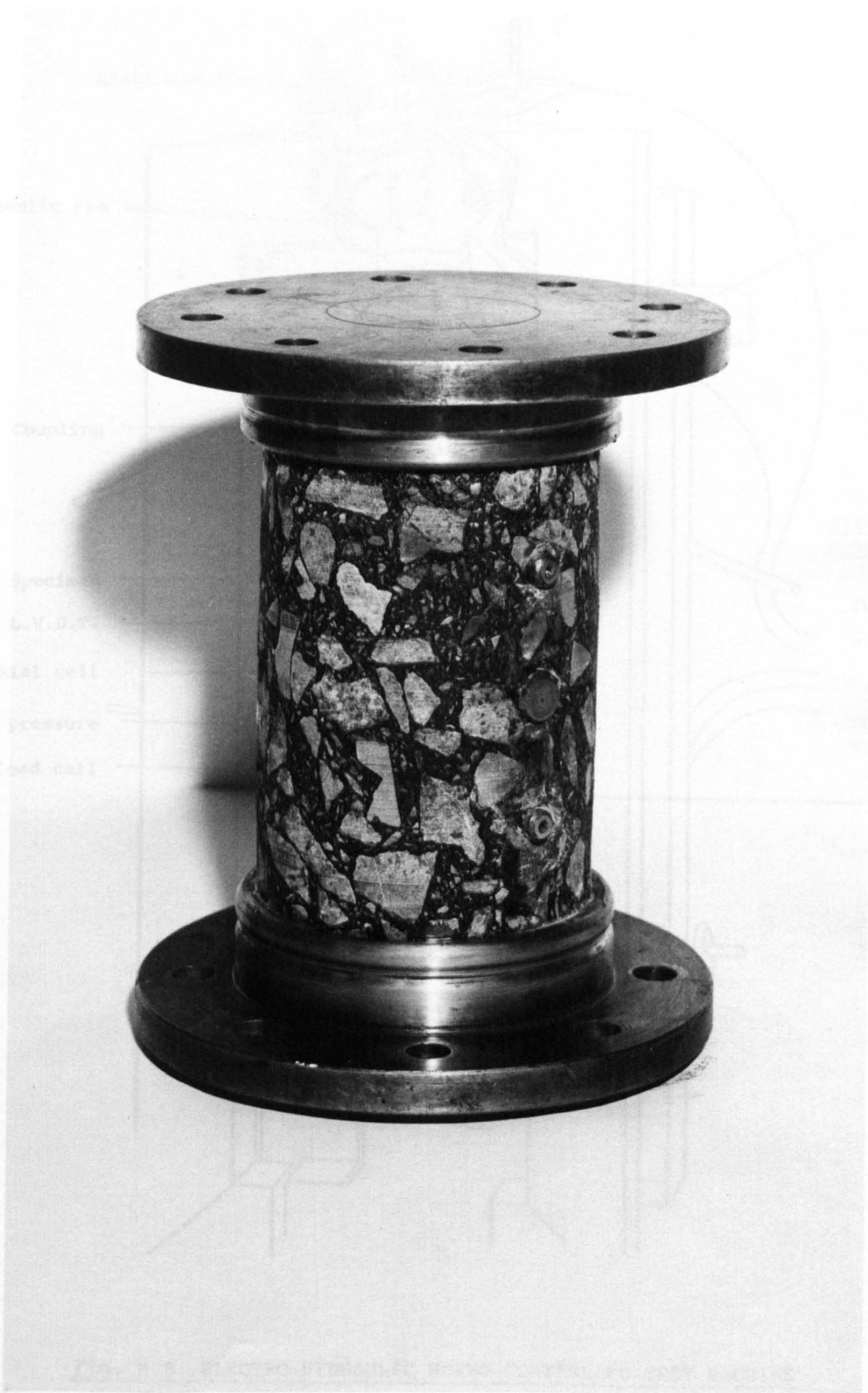
FIGURE 9.4 SPECIMEN WITH LVDT LOCATING PIPS, AND END PLATENS
