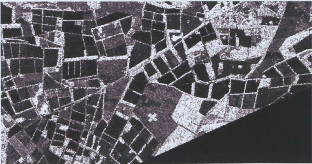
Figure 5.5 SIR-C SAR image containing the study area. The clipping of the image in the lower right corner is due to the limited extent of the SIR-C SAR coverage.
