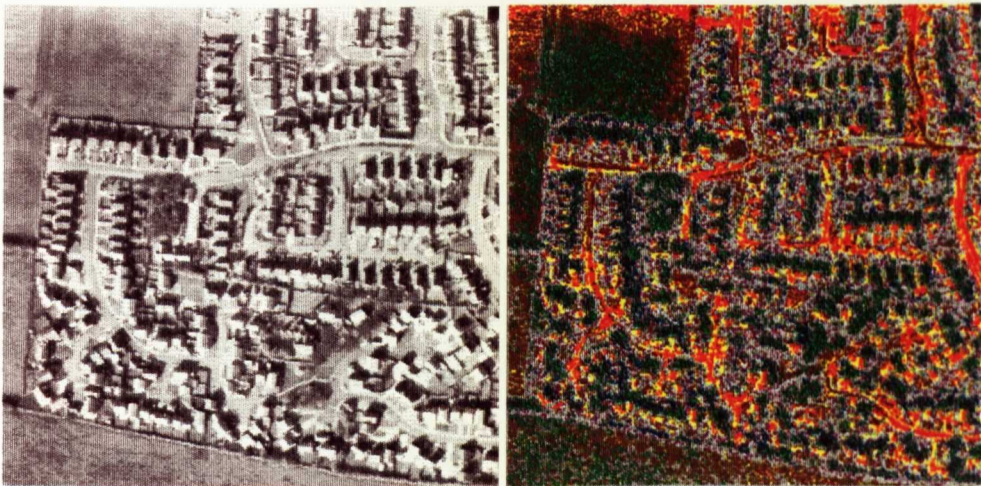
Figure 4.16 False colour image of mean (red), Laplacian (green) and variance (blue) (Z05).
