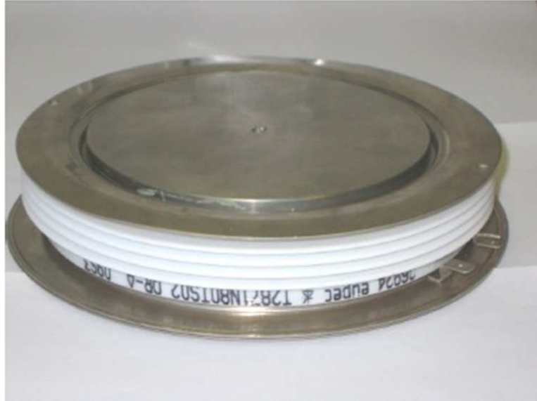
Figure 1.3: A thyristor module (Source: Alstom)
