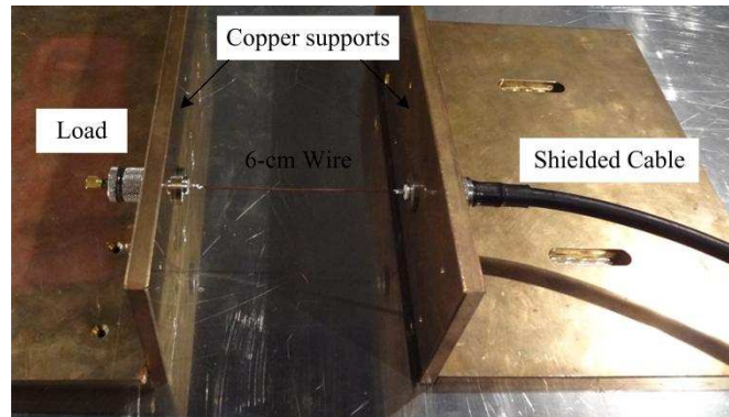
Figure C.1: Short line measurement for the line-end discontinuities characterisation
