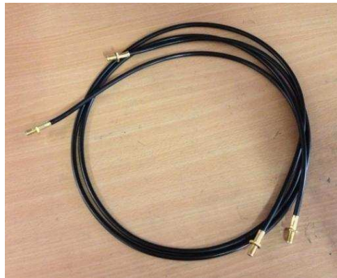
Figure 3.2.1: The two RG-58 coaxial cables with 1.22m in length
