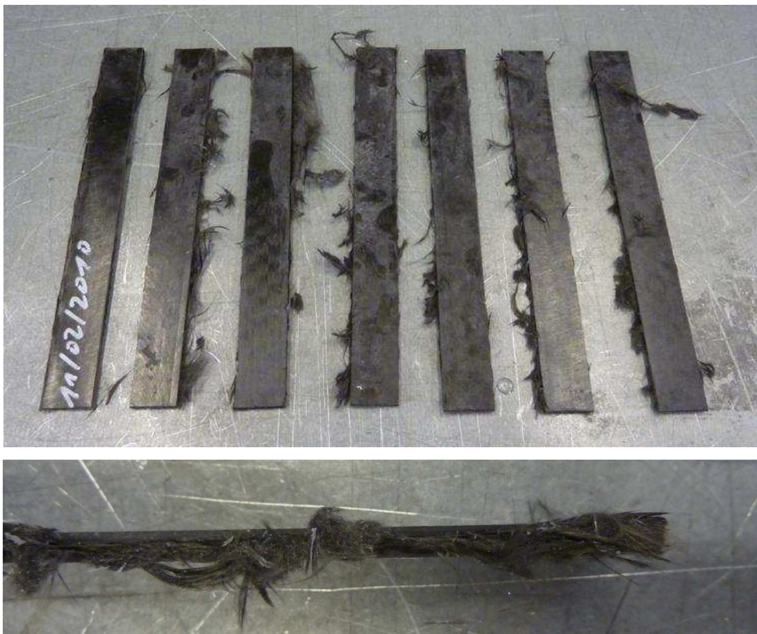
Figure 110. Dry RFPM trial specimens. Although top and bottom surfaces of some plaques looked satisfactory a dry region through the centre resulted in specimens that could not be tested. Plaques were cut by a water cooled diamond saw cutter. As specimens were cut dry fibre clung to the blade resulting in filamentation of any dry fibre tows.
