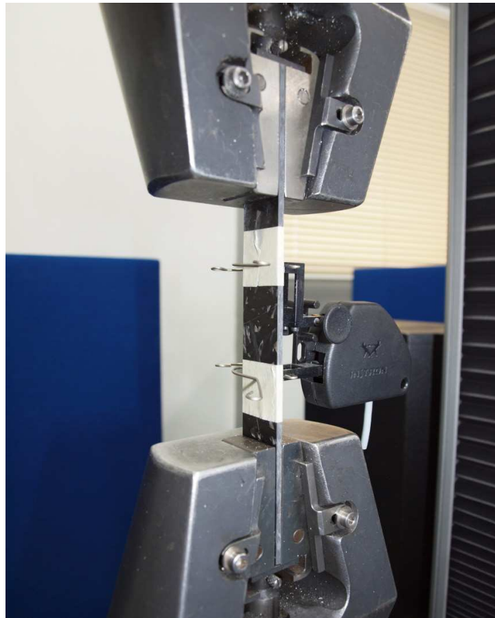
Figure 11. Tensile test. The specimen is loaded into the jaws of an Instron 5581 frame. Two thin layers of masking tape can be seen and were used to prevent slippage of the extensometer.
