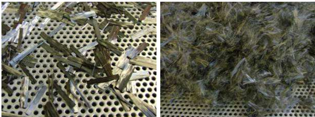
Figure 42. Comparison of highly filamentised 24k tows used by Sotira (right) with unfilamentised tows of the same original bundle size used at UoN.
