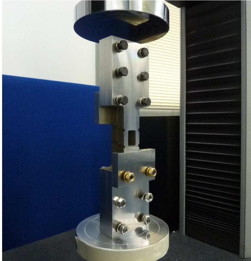
Figure 80. Open-hole compression test rig. Specimens are loaded into the rig with the hole positioned within the central window.
