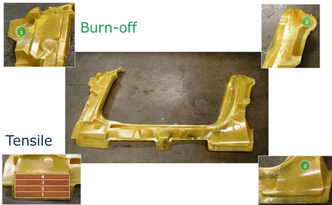
Figure 108. DOR testing plan.
