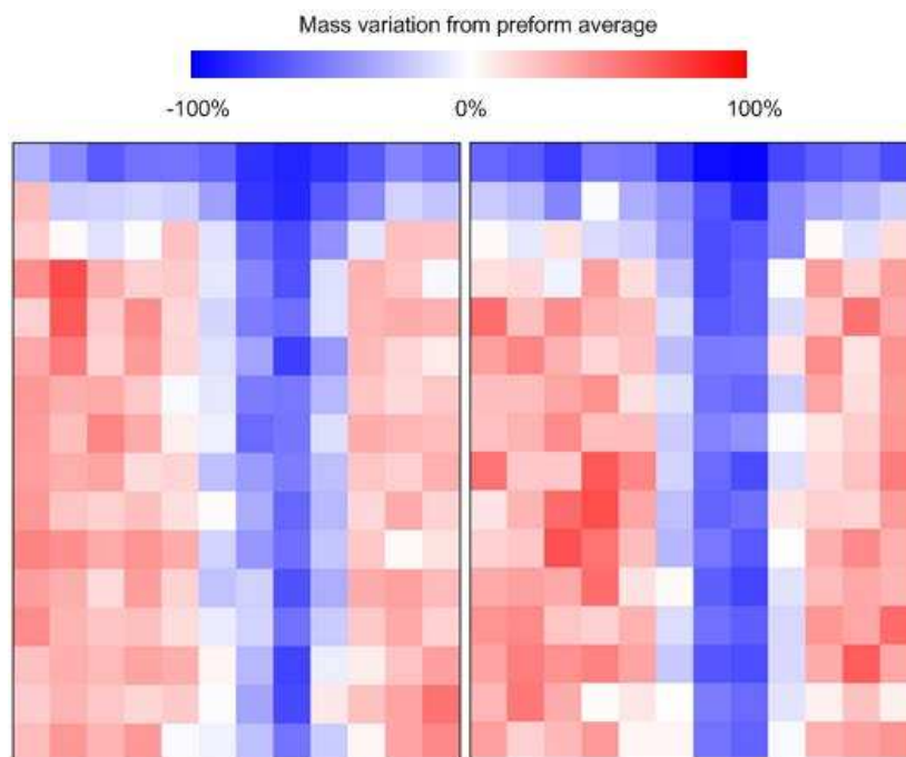
Figure 7-9: Comparison between experimental (left) and predicted (right) mass variability for a preform consisting of 6 K, 30 mm segments with a target areal density of 1.2 kg/m 2 using the robot trajectory in Figure 7-7. TCP height was raised to 350 mm above the deposition plane producing a greater spray cone projection area. This is evident with higher fibre content in the region of the vacant robot path line. The effect of spray bias is also demonstrated with the preform boundary visible along the top portion of the preform.
