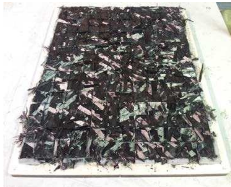
Figure 3-2: Picture of a die cut preform used for process model validation. The preform is cut into 192 coupons of 25 mm x 25 mm dimensions.
