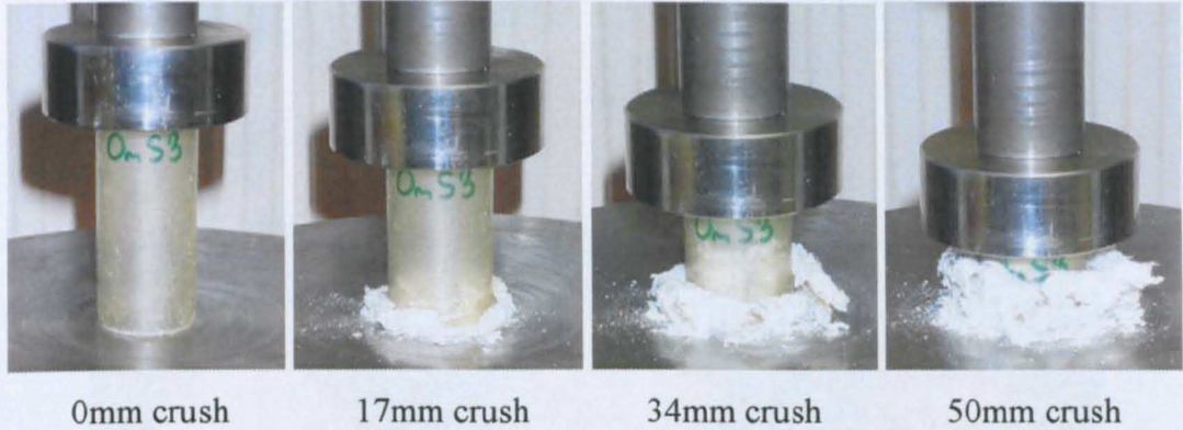
Figure 4-9 – Quasi-static crush of an undamaged, 38.1mm diameter CoFRM/Norpol tube (sample 3)
